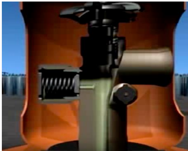
Image: Cut away of a pressure relief valve (source: csb.gov )
