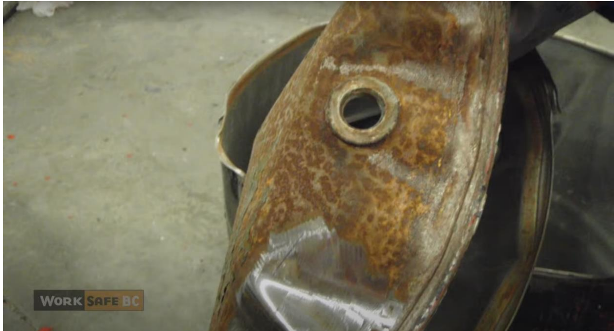
Image: The remains of an exploded drum (source: WorkSafeBC )
